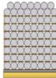
VIEW B: END VIEW WITH NESTED TOP LAYER (TIE-DOWN NOT SHOWN)
